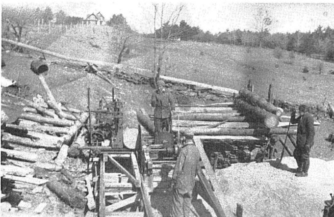
Tischler sawmill: Morris Tischler squaring off a log, Isaac Tischler receiving cut boards, Hillel Tischler with shovel clearing away sawdust from saw blade area.
